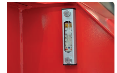
Large oil tank capacity and sight glass.
