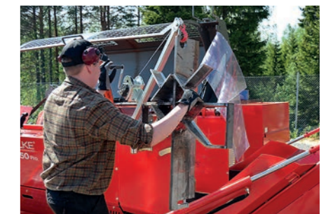
Replacing the splitting blade is fast and safe thanks to the detachable winch.
