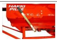
2. Press the lever A to the lower position and then let it return to the initial position.
