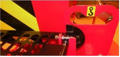
Figure 4. Lifting points for a chain or strap. Translation
