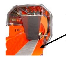
The wood press keeps the logs in place when they are being sawed. Do not put your hand between the wood press roller and the input conveyor belt!
