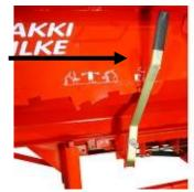
IMPORTANT! Using the machine is strictly prohibited if the splitter's operating lever is in the RUN position and the guard of the splitting section can be opened! The faulty locking mechanism must be repaired immediately. It should only be possible to open the guard of the splitting section
