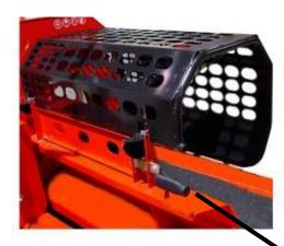
When opening the input conveyor guard, ensure that the locking handle locks the guard in the raised position!
