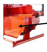
The actual starter box is located behind the splitter, under a protective cover.
