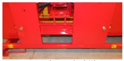
Figure 3. Lifting points for a forklift.
