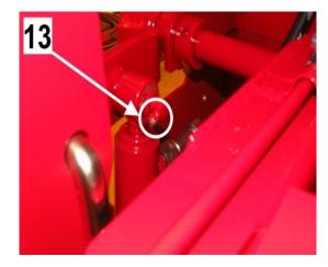
In other words, there is a maximum of 14 lubrication points (Easy model with a pivoting output conveyor). All of the points must be lubricated with vaseline roughly every 10 hours.
