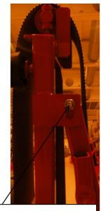
Attach the input conveyor's support (no. 2 Figure 1) to the input conveyor with a bolt.
