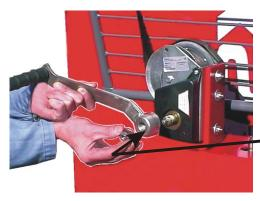
Install the crank for the conveyor winch (no. 8 in Figure 2) by screwing it into place, and lock it with a nut.
