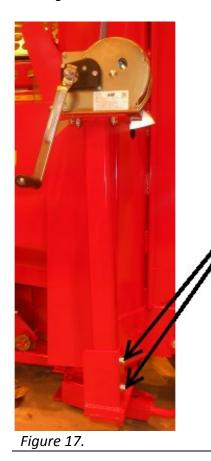
Install the winch support, place the winch (no. 11 in Figure 2) in its slot and tighten the bolts (2 pcs).
