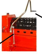
The lever handle can be changed to suit left or right handed users, and the handle can be lifted to the desired height.
