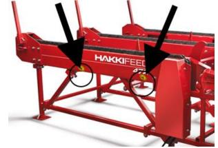
Figure 1. Lifting points of the machine
