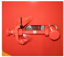
Figure 4 (Adjusting the tightness of the chain conveyor's chains)
