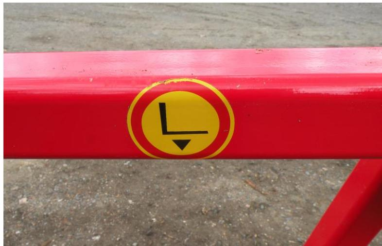
Figure 1. Label indicating the lifting point
