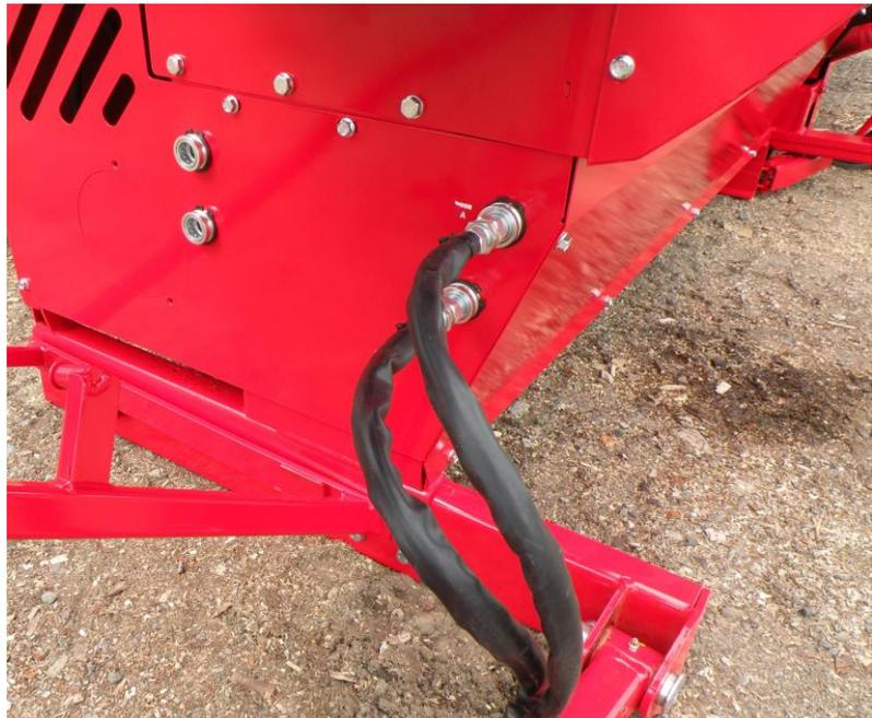
Figure 3. Connecting the hydraulic hose to the machine
