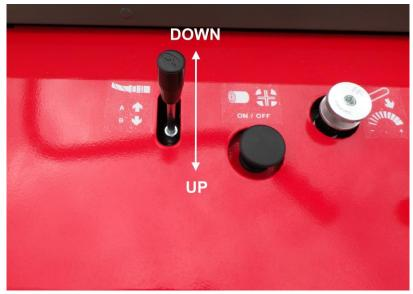
Figure 4. Hoist control lever
