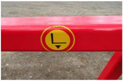
Figure 1. Label indicating the lifting point
