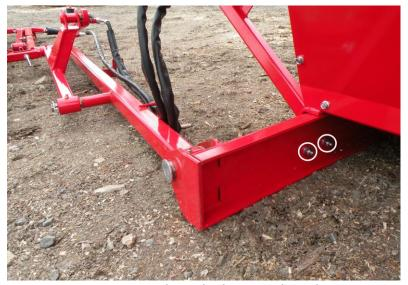
Figure 2. Attaching the hoist to the splitter
