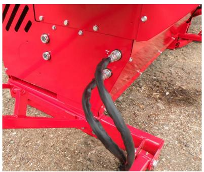
Figure 3. Connecting the hydraulic hose to the machine
