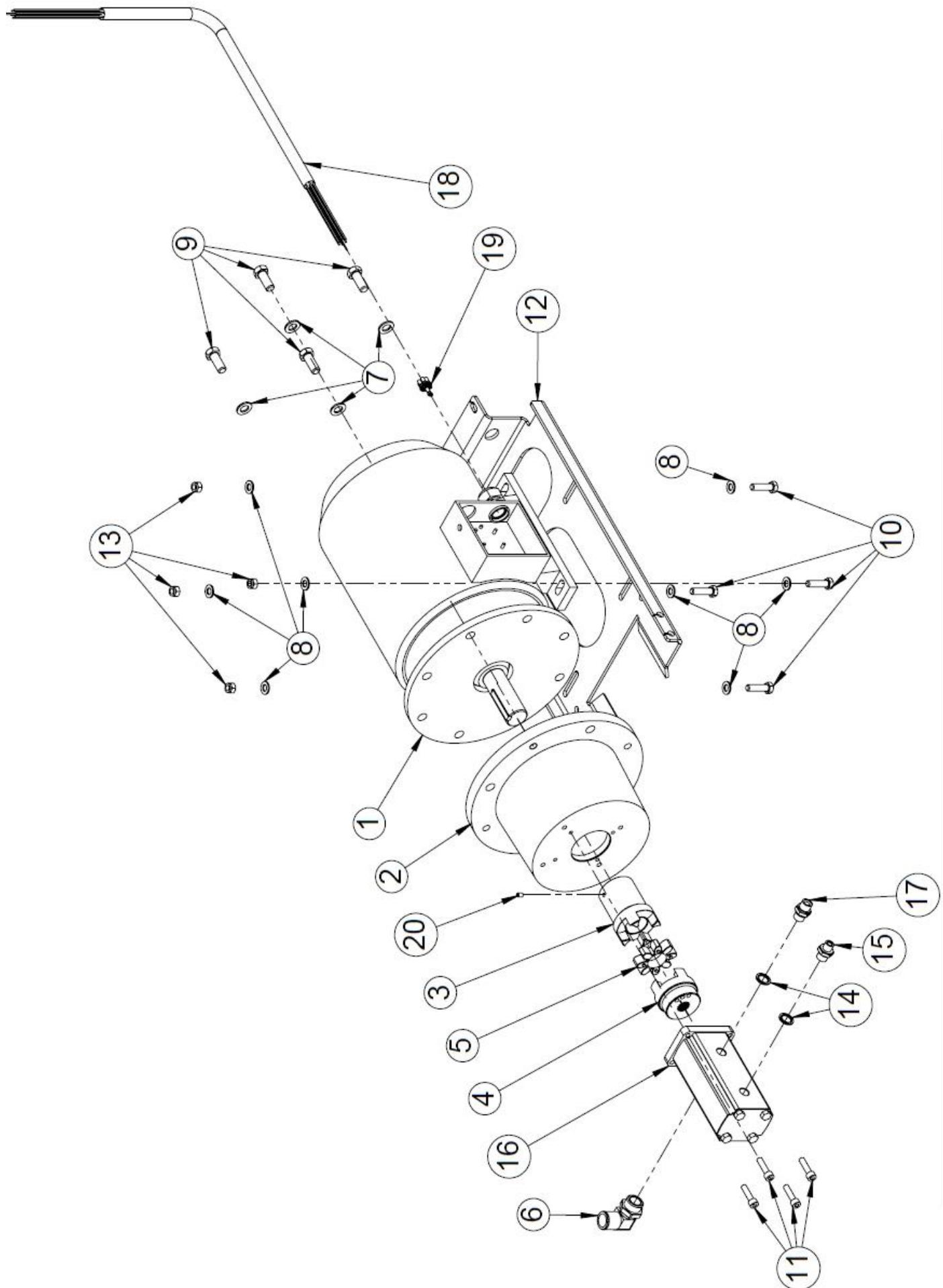
**1.58 Electric motor assembly, 60 Hz/380 V (50036066) parts list**
